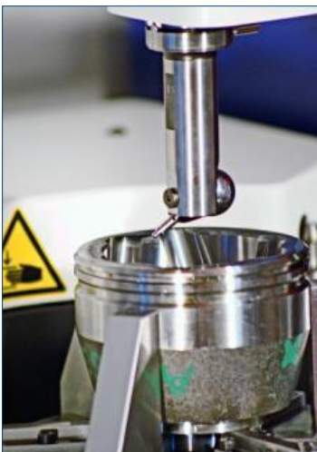
Measuring probe with two different ball diameters for internal contours
